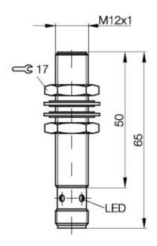
**Inductive Sensors** BES M12MI-POC40B-S04G M12x1 x 65 normally-closed Sn=4mm shielded
